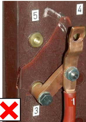
Fig. 9: Surface chipping due to impact on delta connection
