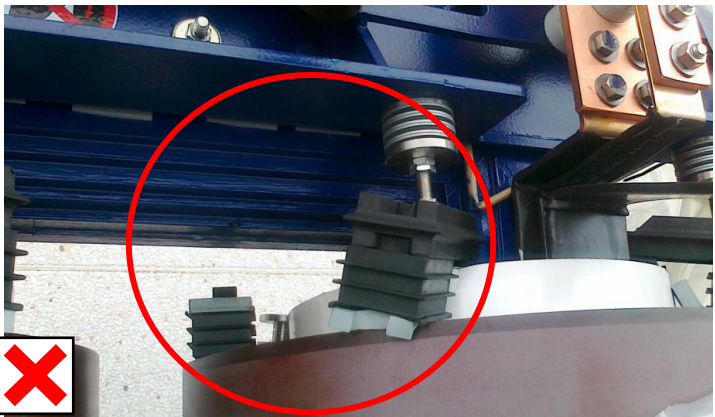
Fig. 12: Windings have been shifted. Recognizable by torn-out or tilting supports.
